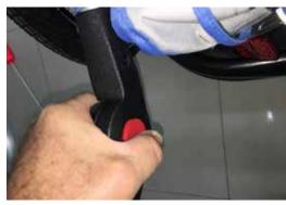
To remove the handlebar, simply depress the spring pin in the upper frame and pull the handlebar off. TIP: Quickest way to remove is one side at a time. Depress the spring pin on one side, then pull slightly until handlebar moves a bit over the release pin, then do same on other side. Finally, pull the handlebar away from the trailer is a slight right-to-left rocking motion to release the handlebar.
