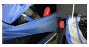
Feed through to the sleeve just inside the rear cabin, adjacent to the frame tube.
