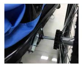
Your Kuji trailer uses simple and convenient push button quick-release wheels. To install the wheel, first push the button on the outside of the wheel hub, and insert the axle through the hanger bracket on the frame as shown. Push all the way in and release the pushbutton. The wheel is automatically locked in place. Give each wheel a tug to make sure they are secure.
